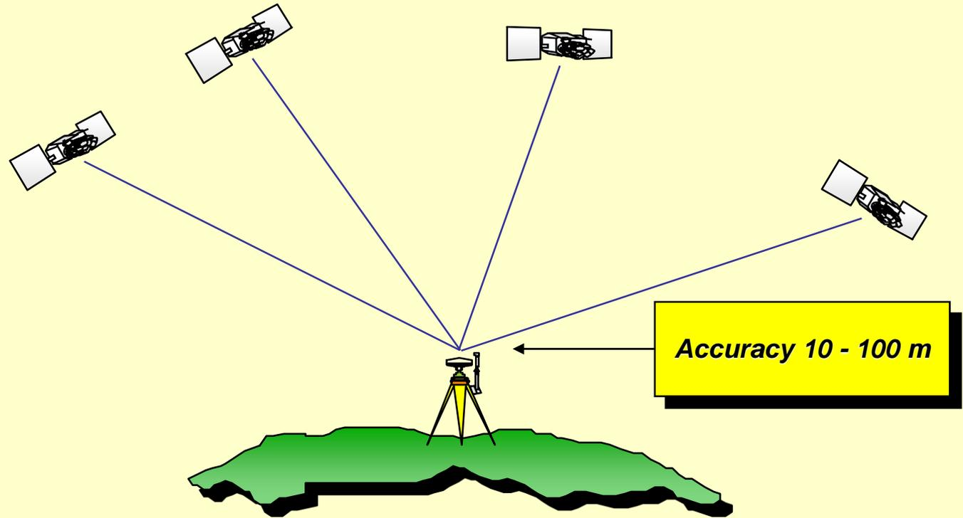
A receiver in autonomous mode provides navigation and positioning accuracy of about 10 to 100 m due to the effects of GPS errors!!?
