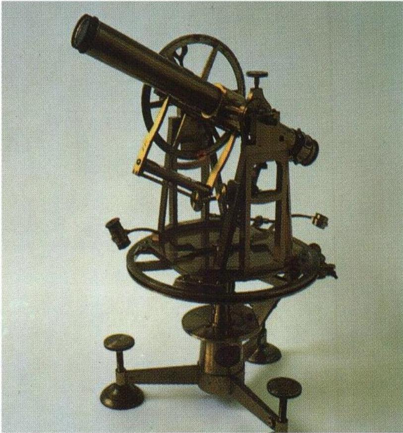
Theodolite is designed to measure horizontal & vertical angles accurately.
